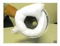
**Step 8:** (**Fig 17**) If the packing pillow begins to bunch up, you may need to use a flat head screw driver or a ruler to push down the bunched up packing. Be sure to correctly align the core so that it fits over the inlet cap at the bottom of the muffler.
